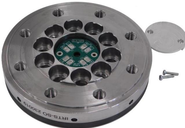
Figure 15 IRTS-P Tempdisc: Rotor without cover
