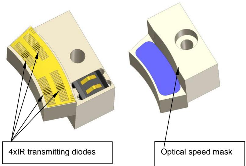
*Figure 5-7 Speed measuring adjustment*
