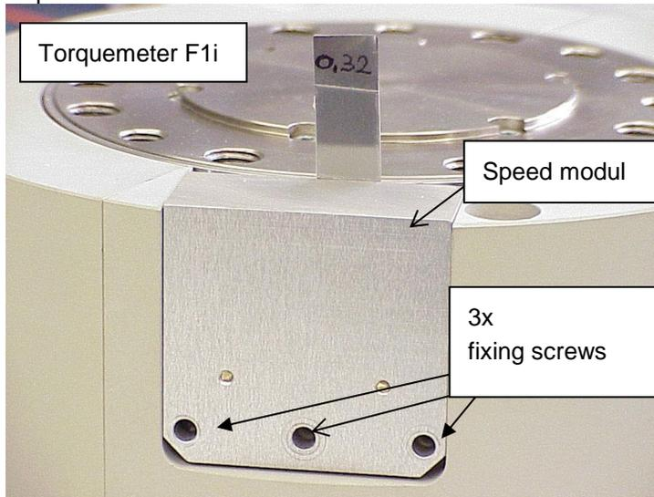
Figure 5-3 Adjustment of speed measuring
