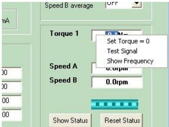
Figure 8-3 Torque zero adjustment
