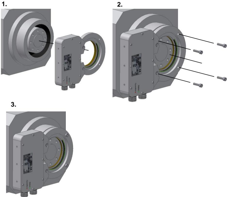
Figure 4-18 Mounting the stator
