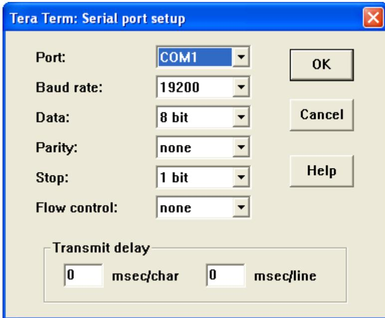
Figure 11-3 Tera Term: Serial port setup
