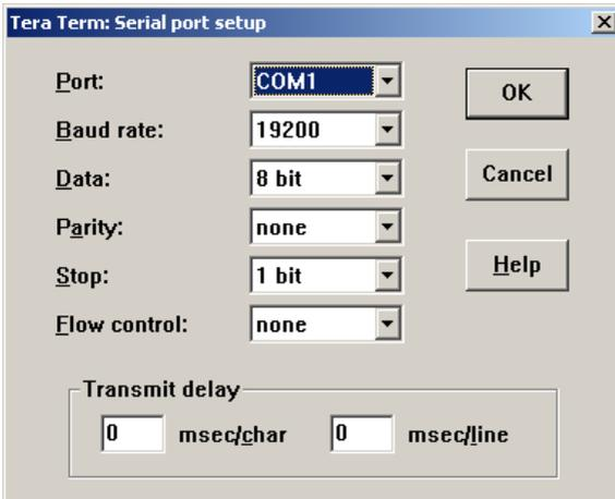
Figure 7-4 Tera Term: Serial port setup
