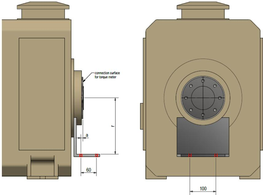
Figure 4-5 Mounting to angle plate
