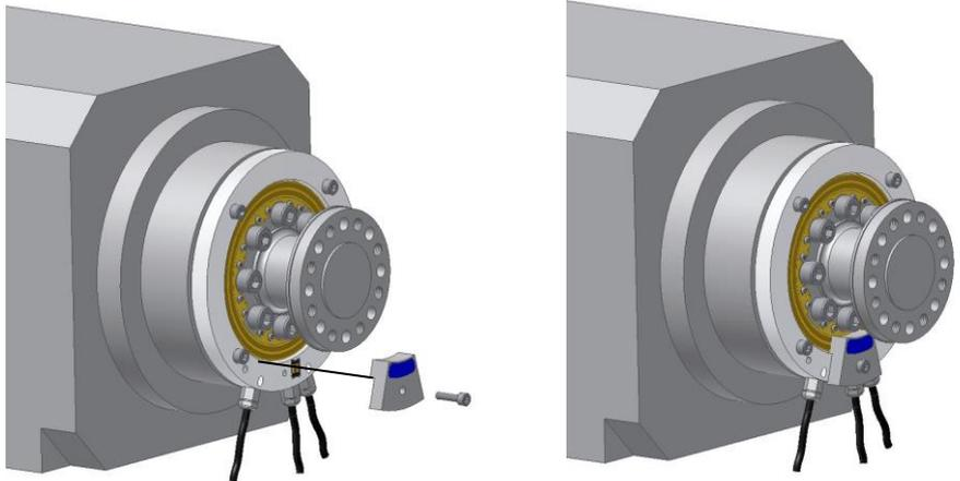
Figure 4-31 Mounting optical speed detection
