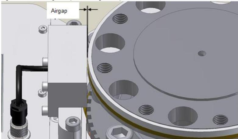
Figure 4-10 Air gap between speed measuring system and measuring flange (see Chapter 5 Speed measuring system)
