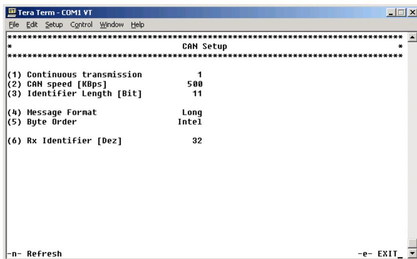
Figure 8-19 CAN set up
