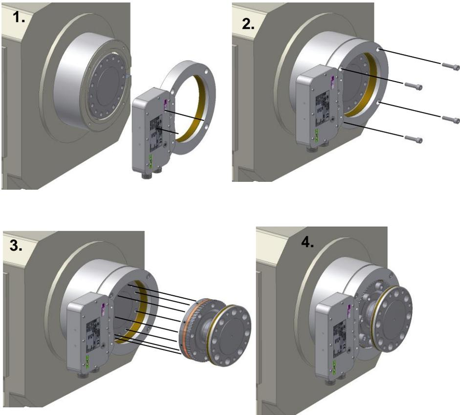
Figure 4-2 Mounting of the stator
