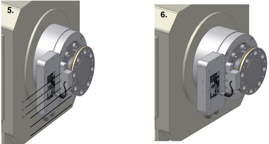
Figure 4-9 Mounting the optional magnetic speed detection
