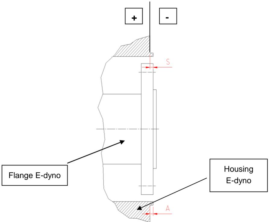
*Figure 4-14 Offset between flange and housing*
