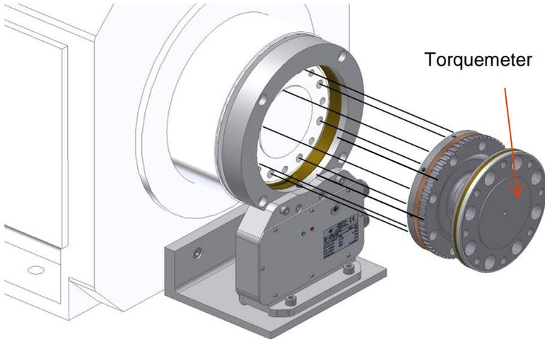
Figure 4-6 Mounting of torque meter
