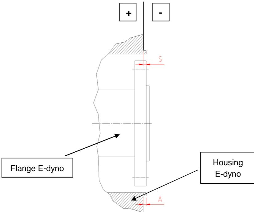
Figure 4-1 Offset between end faces (dynamometer flange/dynamometer-housing)
