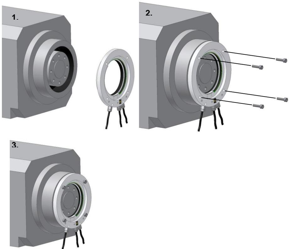
*Figure 4-28 Mounting the stator*
