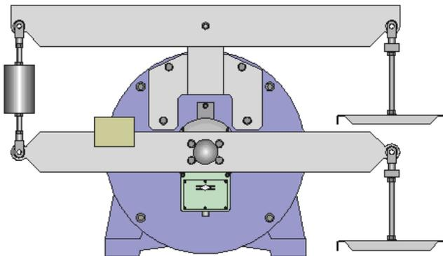
Figure 14-1 Calibration system
