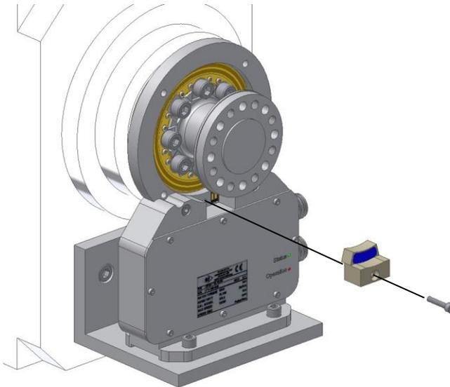
Figure 4-26 Mounting optical speed detection
