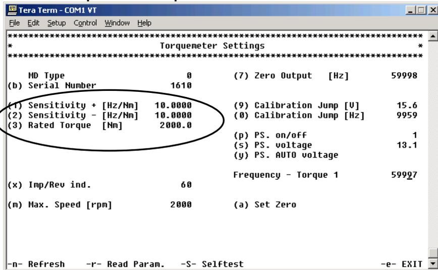
Figure 7-5 Setting calibration parameters
