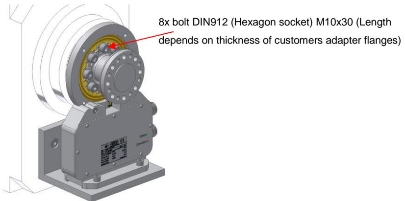
*Figure 4-24 Mounting torquemeter*
