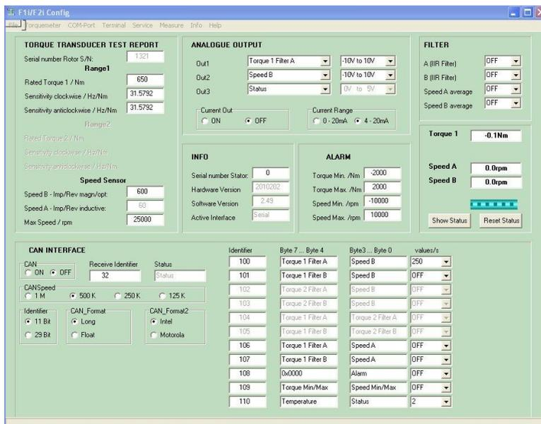
Figure 8-2 Settings after selecting correct port
