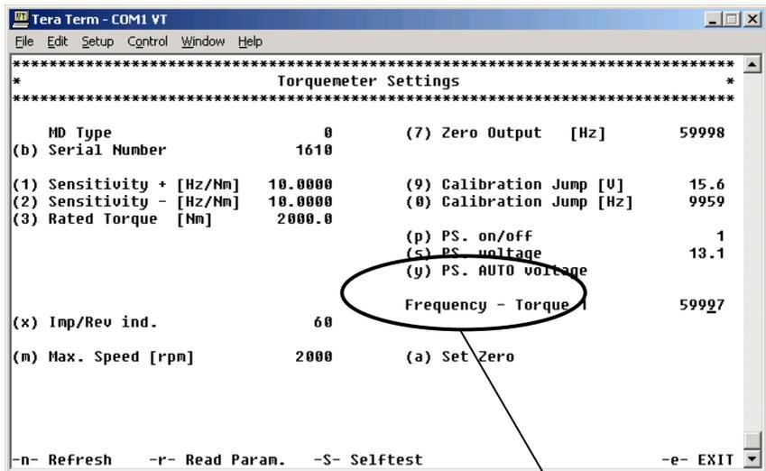
Figure 7-6 Automatic inductive power supply adjustment
