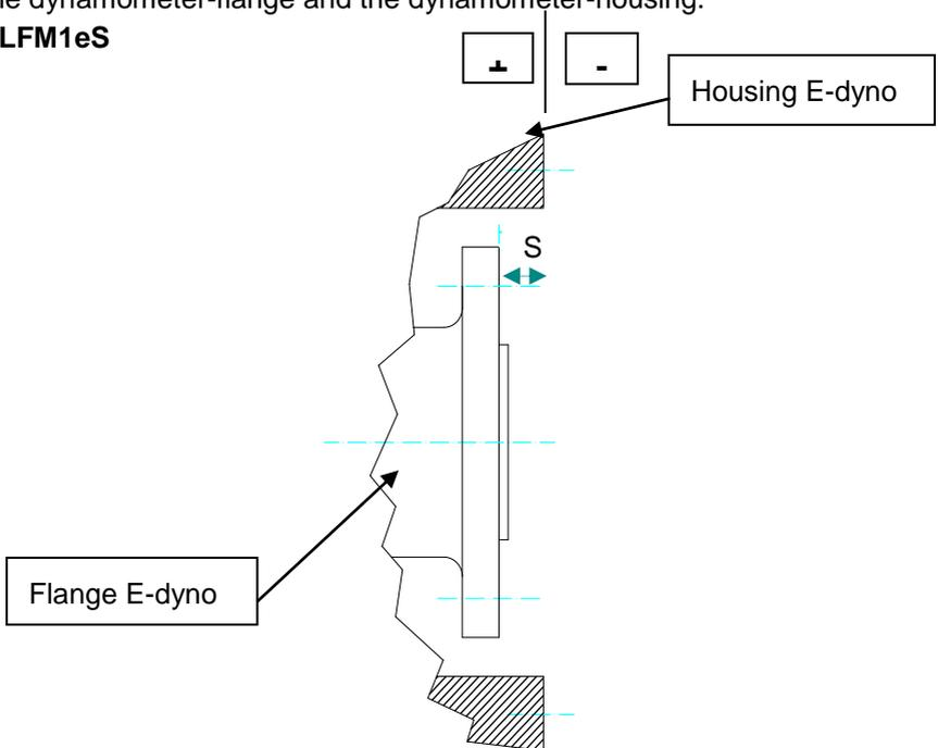
Figure 4-27 Correct offset between house flange and housing
