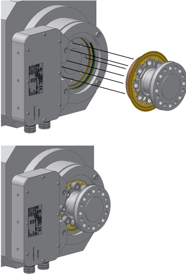
Figure 4-20 Mounting the rotor
