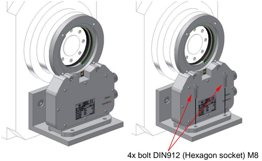
*Figure 4-23 Mounting stator with foot base*
